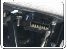
2. Connect the male end of the included plug-n-play HWK-TW01-HAR to the vehicles factory ODB II connector. 3. Secure the OBD II connector and the harness together using one of the included wire ties and cut off any excess wire tie that is not needed.
