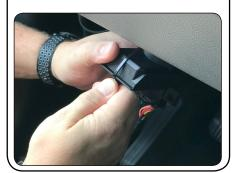
4. For the Nut and Bolt style mounting system: Place the ears of the connectors over the factory studs and replace and tighten the fasteners removed in step 1. Use the included self tapping screws to secure if this connector is not a factory fit. For the clip in style mounting system: Feed the body of the harness into the dash opening and secure connector to the dash using the included self tapping screws.
